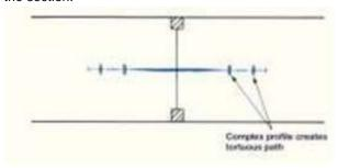
The Expanbar\* range incorporates both of these principles. The products offer a fully continuous 4 bulbed design maintaining both the valve and tortuous path principles. These principles are maintained in the transition from Rearguard profiles in floors to centrally placed profiles in walls.
